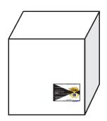
2. If the package is twice as long as it is wide, use two ShockDot impact indicators. Place a second indicator in the same position on the opposite side of the package.
